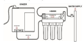
**Step 4** :: Connect hosing to the outflow port on the Stage 3 side of the system.
